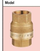
**HERZ** spring check valve Body of brass, EPDM seals, spring of stainless steel. Opening pressure: 0.02 bar. Temperature range from -10°C to +110°C.
