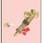
**ERZ Strainer** with draining valve, fine-mesh strainer chromiumnickel steel, body of dezincification-resistant brass - socket x socket.
