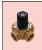
Four-way mixing valve, female thread, body and cone of 15 1 **2138** 01 brass, EPDM seals, medium temperature -10°C to 120°C. Actuator of choice 1 7712 25/27 to be ordered 20 1 **2138** 02 separately.
