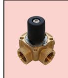
Four-way mixing valve, female thread, body and cone of brass, EPDM seals, medium temperature -10°C to 120°C.
