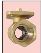
HERZ two-way ball valve with female thread, for precise regulation, no leakage losses, regulating ball valve for continuous control of cold water, warm water in closed circuits, pressure level PN 40 (DN 15-DN 25) or PN 25 (DN 32-DN 50), ball with equal percentage characteristic graph, spindle sealing with double O-ring, actuator of choice 1 **7712** 33/35 to be ordered separately.
